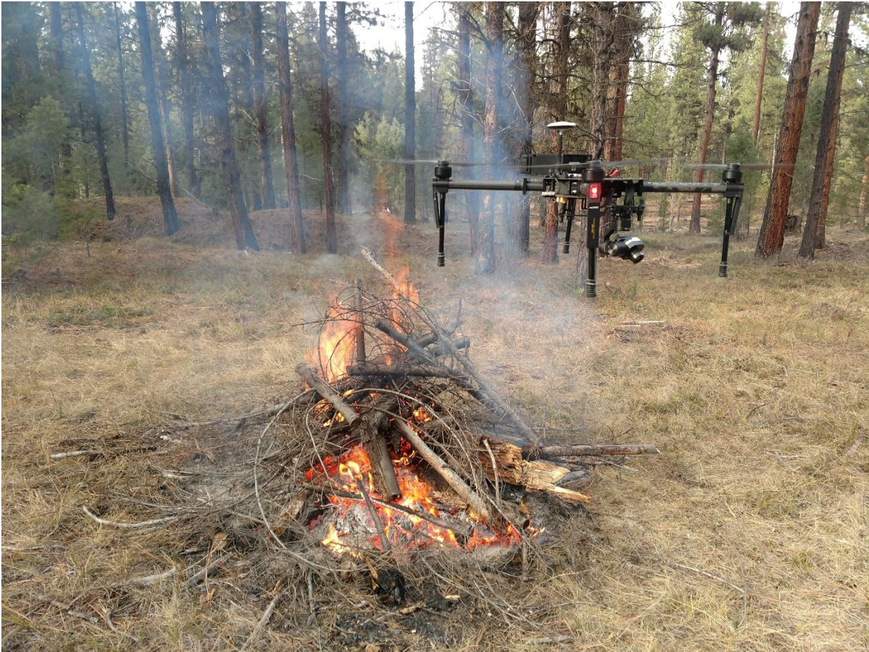
Calibrating thermal camera on burning slash piles at Lubrecht Experimental Forest.
