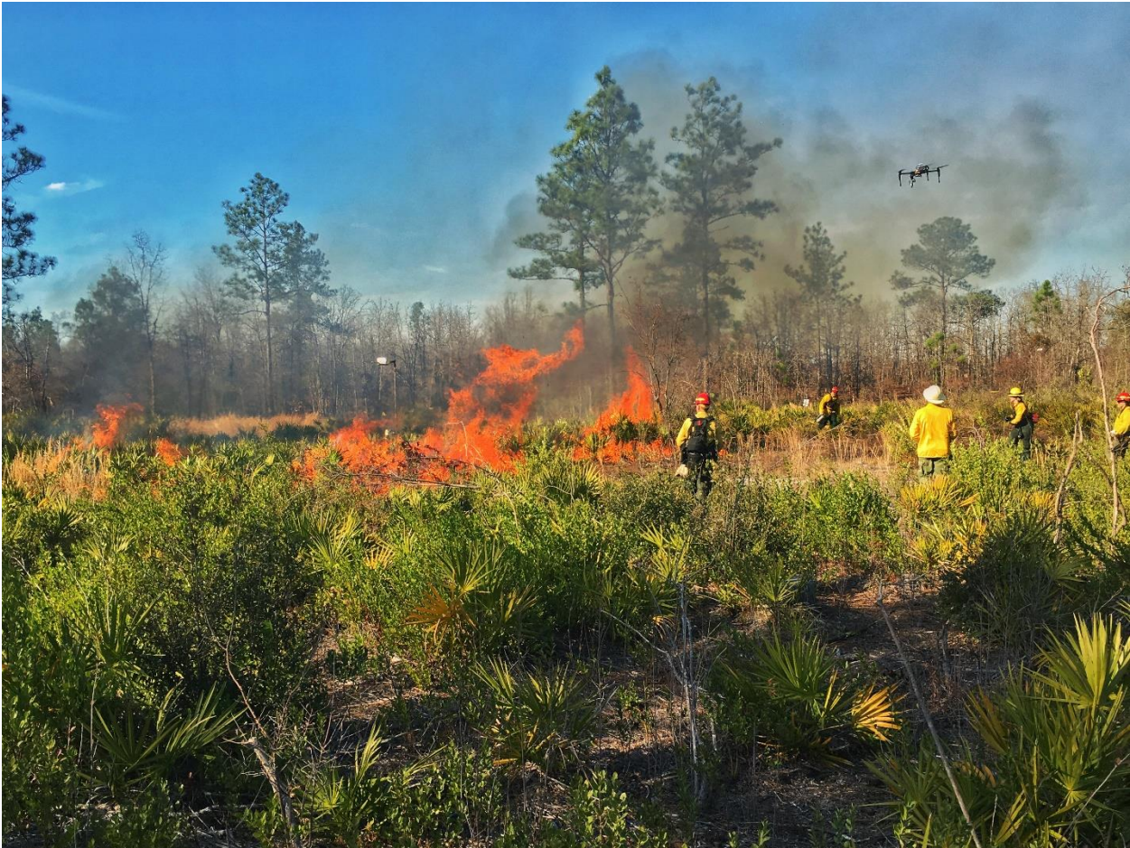
Researchers collecting coincident in situ and drone-based thermal data. Sensors in the fire are being used to calibrate thermal imagery from the drones.
