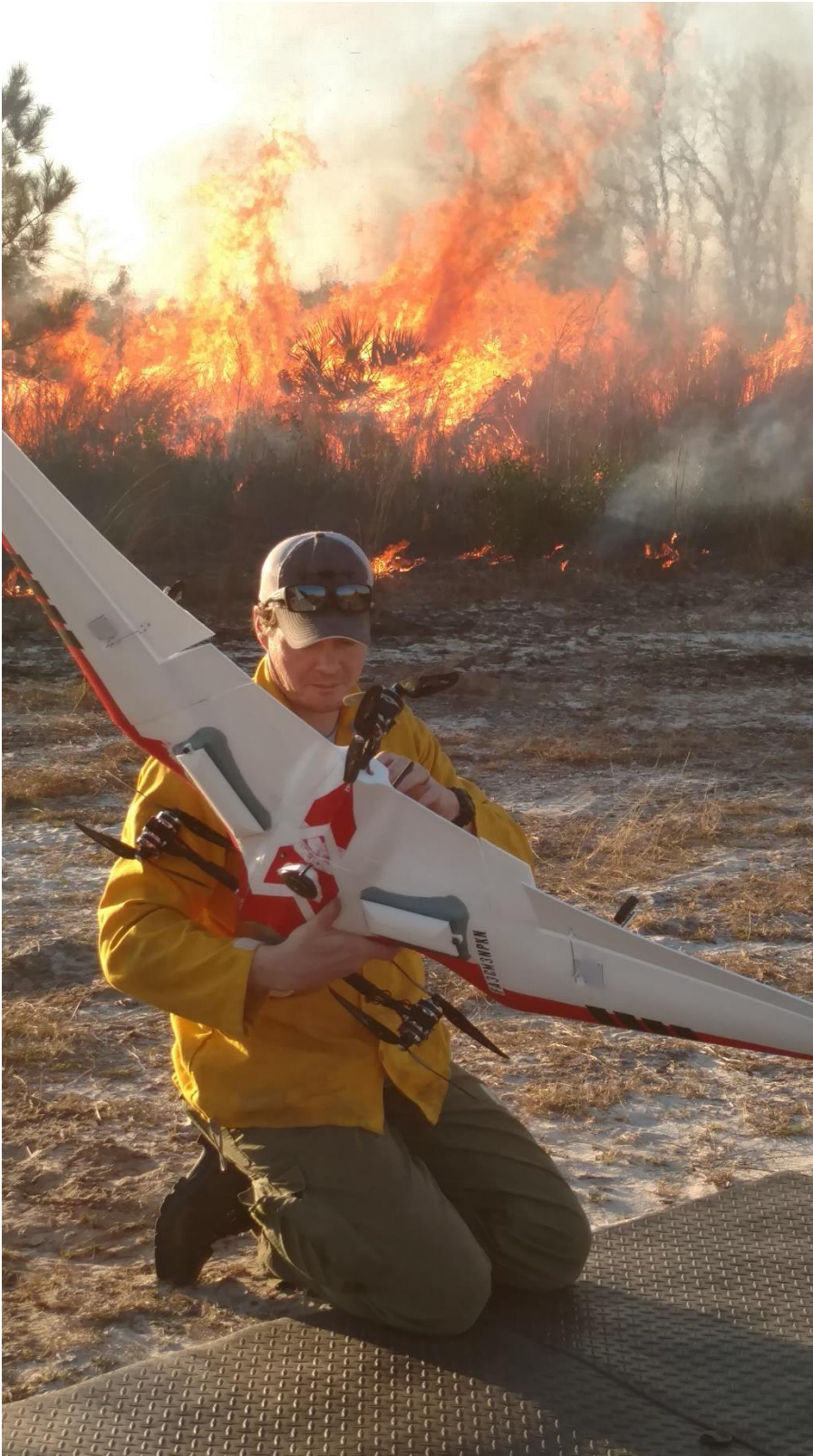
DroneFire technician preparing vertol FF6 platform for launch on prescribed fire in Georgia.
