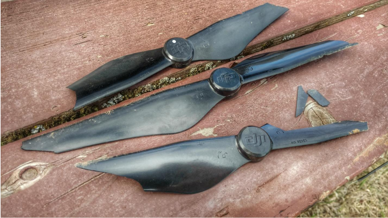
Steep learning curve - broken rotors after test-flight.
