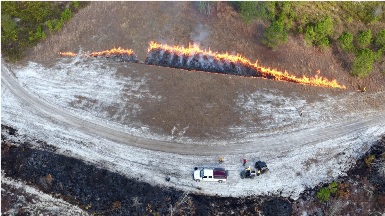
Researchers light ignition strip to carry fire into highly instrumented field plots. Drones are being used to characterize thermal energy from multiple look-angles and elevations.
